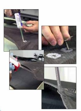
Permabond ET500 is used to bond fasteners to a carbon fibre car bonnet and Permabond PT326 bonds the 2 skins of a carbon fibre car bonnet together.
