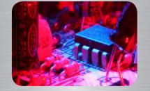
Soldering and fixing components to either side of a PCB can be very difficult - when you try to solder one side, the component drops off the other. Permabond adhesive can be used to secure components which may later need to go through a solder reflow process.
