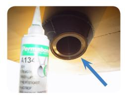
This particular customer was unable to weld cast iron to steel and decided to bond the rudder bushing in place instead. Less accurate machining of parts was required as the high viscosity adhesive was able to take up the slack fit between parts.
