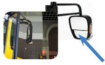
Toughened, impact resistant adhesives for bonding vehicle mirrors to ABS. It is vitally important the adhesive has flexibility to cope with differential thermal expansion and contraction and a high level of vibration
