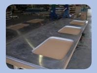
Securing exterior panels or "skins" to buses, coaches, trains etc with old fashioned screws and fasteners is now a thing of the past. Nowadays for a seam-free, streamlined exterior, manufacturers are opting to use adhesives for joining panels to framework. Not only is it a requirement that the adhesive be strong, toughened and able to withstand vibration and impact, it is also essential that shrinkage is minimal during adhesive cure so as not to show witness marks through thin skins.
