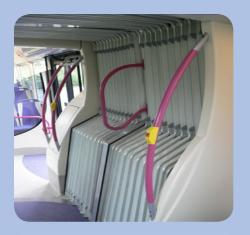
Bellows (the accordion part) on bendy buses and in between train carriages are often bonded with Permabond POP primer and a cyanoacrylate.
