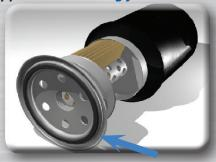
Rolled seams are found in oil filters, fuel filters and air filters. They are formed by cold rolling the edges of two metal flanges like the lid of a tin can. Generally the "can" is rotated while a stationary set of rollers moves in to crimp the can closed.
