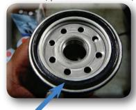
beverage filters. In oil filters, cyanoacrylate adhesives are generally used to bond the gasket to the outside of the base plate as they offer a rapid cure speed and are oil and gasoline resistant. This gasket helps to seat the oil filter properly when it is installed on the engine.
