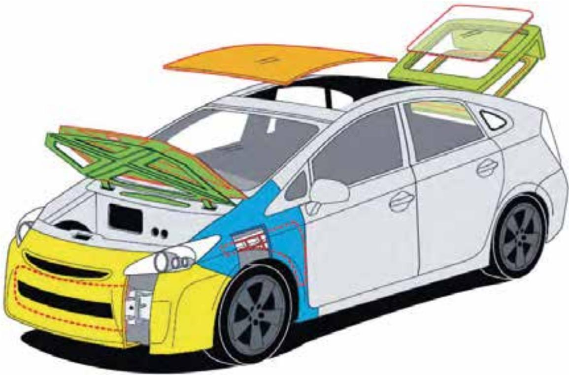
**Figure 2** Potential application areas of bonded hybrid composites
