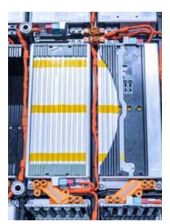
Electric vehicle batteries need thermoregulation to protect battery performance and lifespan. With demands for faster charging rates and higher, consistent battery performance, dependability of the thermal management system is critical.
