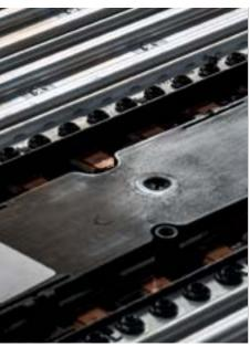
Due to temperature swings, the screws securing the coolant system to the battery pack made noticeable noise during expansion and contraction.
